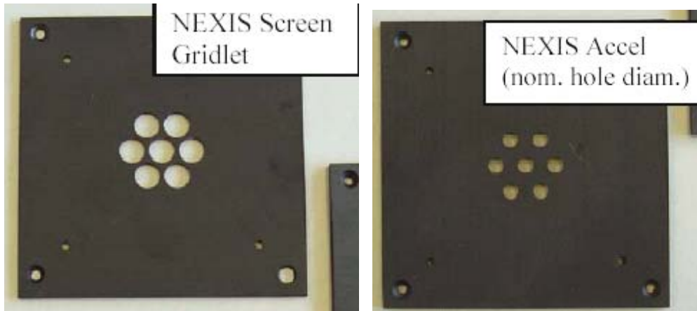
Figure 3.45 Photographs of NEXIS gridlets fabricated from Poco graphite.
